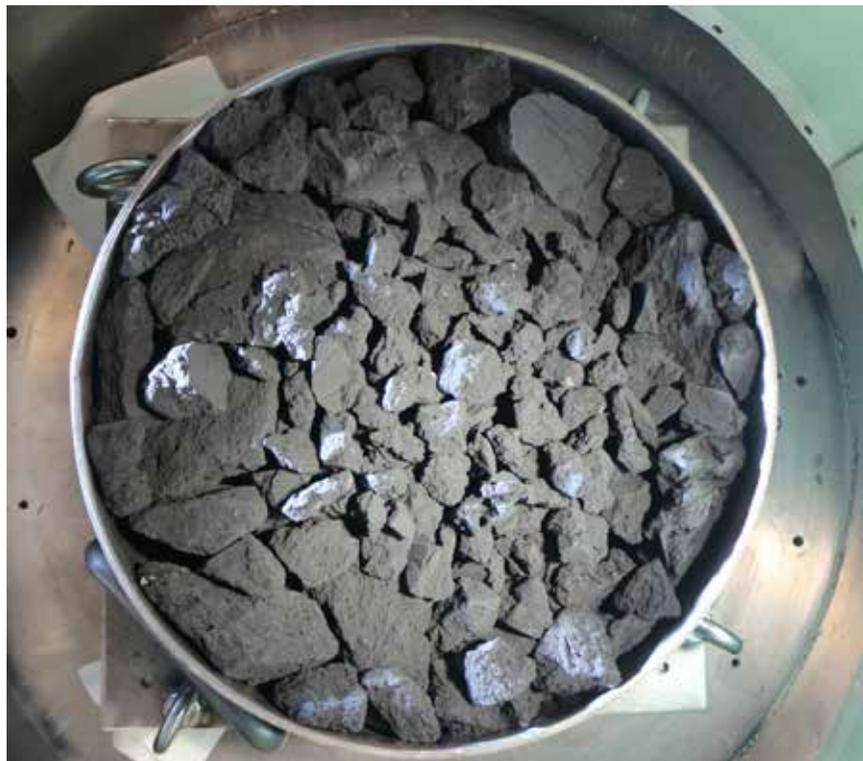
Target simulating the surface of Ryugu.
