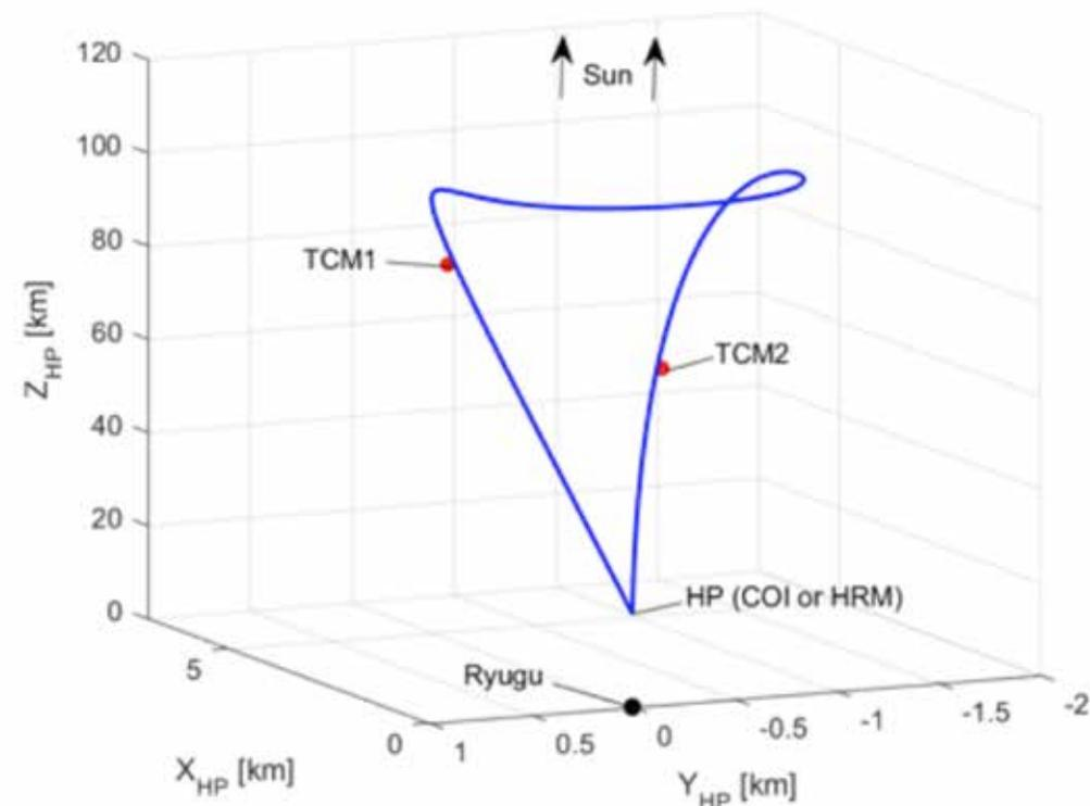
Transition orbit during solar conjunction in the home position coordinate system
